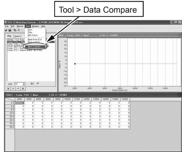
Fig. 26: Data comparison dialog startup
